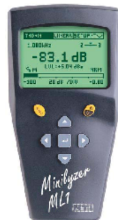
MiniLyzer ML1, can be upgraded to STI-PA functionality
